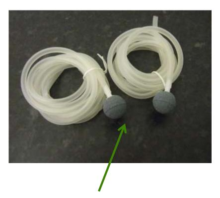
The airstones simply push fit on to the air line as shown above
