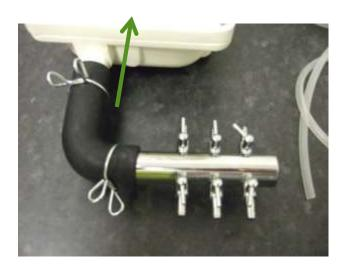
The manifold holder fits over the single air tube fitting holder. To the other end the manifold is pushed on and both ends are securely fitted via the provided clamps.
